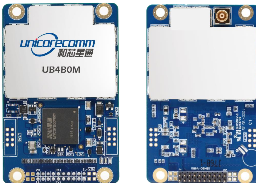
Figure 1-1 UB4B0M All-constellation All-frequency Compact High Precision Board
